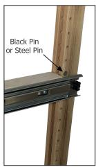
Set the 2nd set of Drawer Rails on the 3rd pin hole above the box just placed. Remember to add a pin above the Drawer Rail on the back upright to prevent the drawer from falling when it is pulled out. Use either the steel pin or gold pin depending on your access to the upright.
