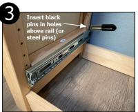
After the steel pins are set, insert Left and Right Drawer Rails to sit on top of the pins. IMPORTANT: Insert a steel pin above on the rear upright for each Drawer Rail. INSERT THE TOP STEEL PIN FROM THE OPPOSITE SIDE OF UPRIGHT. Or use our Black pins that are thinner and will be easier to slide over the drawer suspension. VERY IMPORTANT: These pins will prevent the drawer from falling when pulled out.
