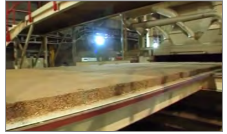
Wood chunks are baked into panels
